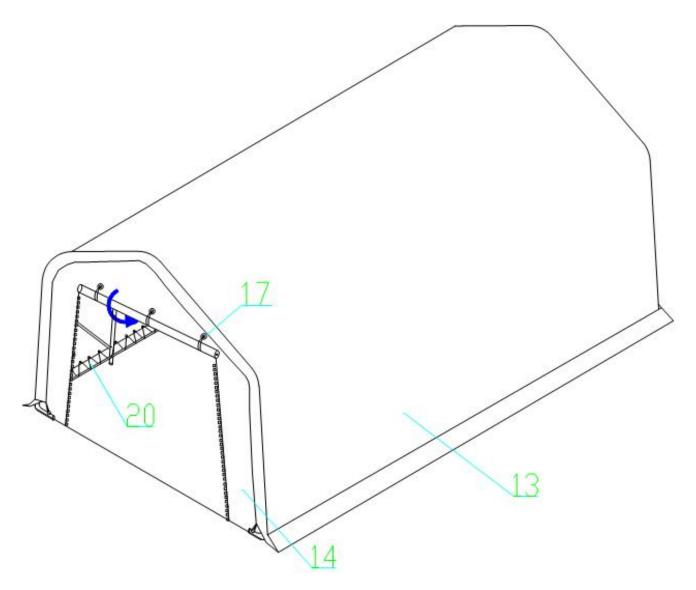
**3.** Knit the Roof Cover and the Lowest Horizontal Connecting Tubes by using the Rope (part No. 20).
