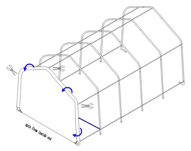
1. Put on the Front Door cover (part No.14) from the inside of the door frame to the outside and
