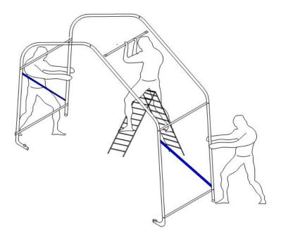
2. By turn, connect the other group arches by using Male Horizontal Connecting Tube (part No.5) and Bolt M8\*80mm (part No.15) Please make the Horizontal Connecting Tube under the arch frame, the roof cover could be supported beautifully.
