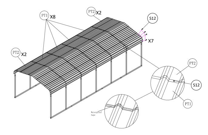
NOTED: Both end of Panels PT1 have holes, Please noted the short holes space are connect with Panels PT2.
