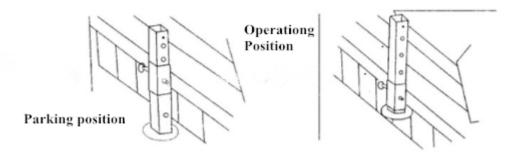
ATTENTION! Prohibit to be in the space between the machine and the tractor, when we change the machine from the position of placement to the position of working
