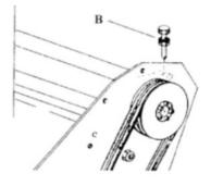
Before using, tighten all bolts, all nuts and all screws
